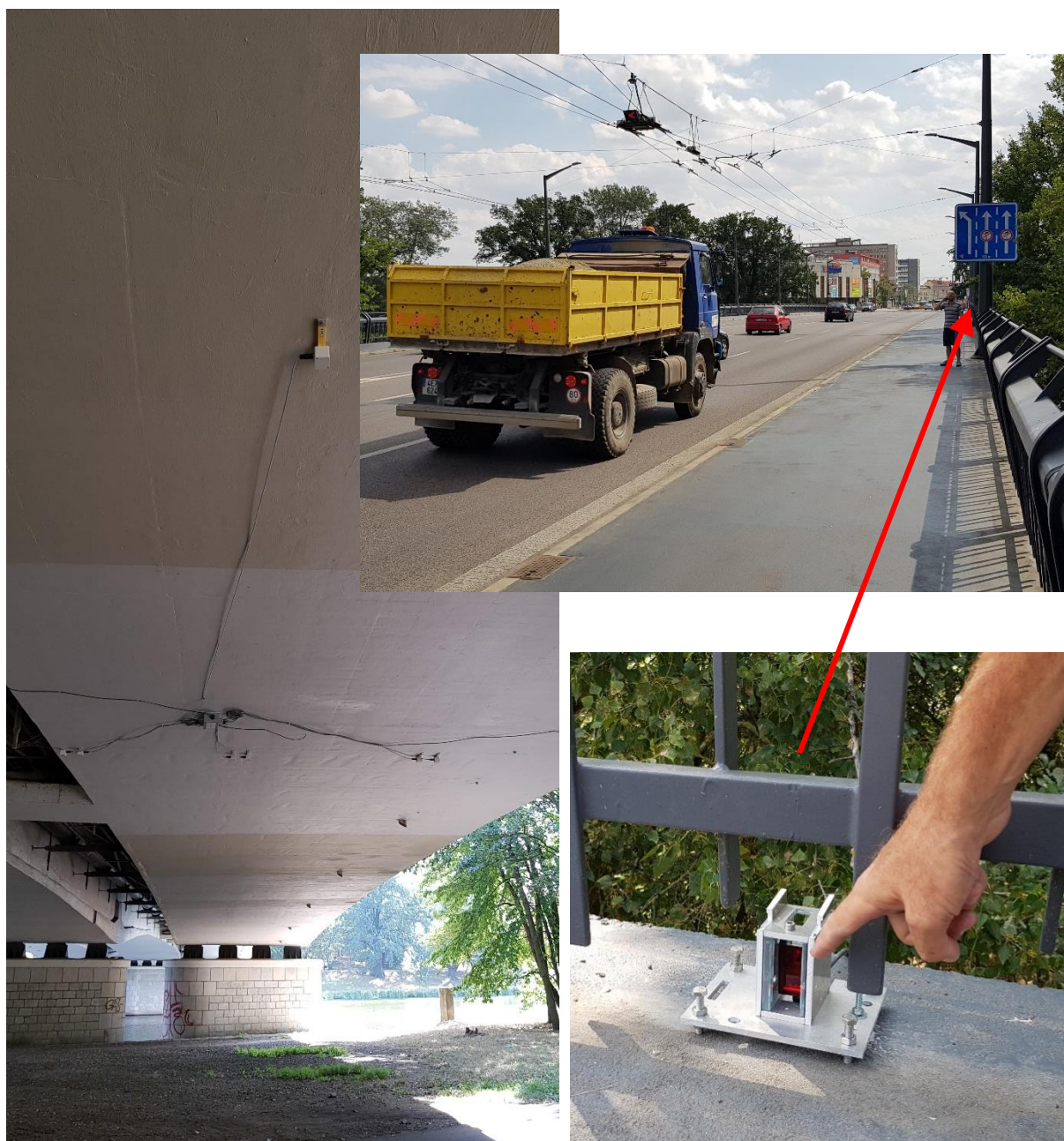
Fig. 2-4: Monitoring installation (left) on Wonka bridge in Pardubice, calibration using trucks with pre-defined weight (top right), laser sensor for detection of vehicles, their location on the bridge and axle distance
